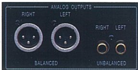
Analog outputs also accommodate balanced connections.
