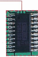
20-bit D/A converters (six units on rear side)
